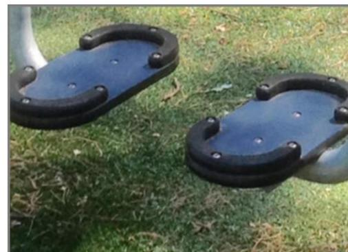
Pedals are constructed of hot-dip galvanized steel with a pedal plate made of Ekogrip® panels of 0.59" polyethylene with a 0.12" top-layer of thermoplastic rubber. This provides a non-skid effect for comfortable and safe training at all weather circumstances.
