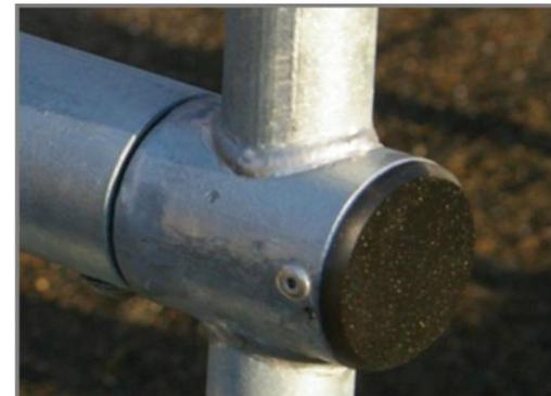
Bearing unit is constructed of hot-dip galvanized steel with a stainless steel AISI 304 shaft and two ball bearings. This will provide a smooth movement, even in the toughest circumstances.
