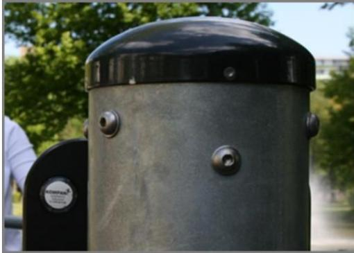
For ensuring the integrity of the main frame the support post is made of a hot-dip galvanized steel tube of 6.3", with a wall thickness of 0.16" and has a post cap made of powder-coated aluminum.
