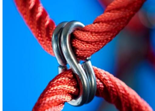
Corocord 'S' clamps are used as universal connections in Corocord products. .31" stainless steel rods with rounded edges are pressed around the ropes with a special hydraulic press, making them the ideal connector: safe, durable and vandalism-proof, all while allowing the typical movement of rope play structures.
