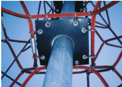
Corocord membranes consist of friction-proof rubberized material of conveyor belt quality with excellent UV resistance. Tested and compliant with REACH requirements for PAH. Embedded is a four-layered armoring made of woven polyester. The armoring and the two surface layers result in a total thickness of .29"
