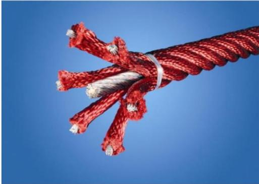
Corocord ropes with .75" diameter or more are special „Hercules“ – type with galvanized six-stranded steel wires. Each strand is tightly wrapped with PES yarn, which is melted onto each individual strand. The ropes are highly wear- and vandalism-resistant and can be replaced at site if needed.
